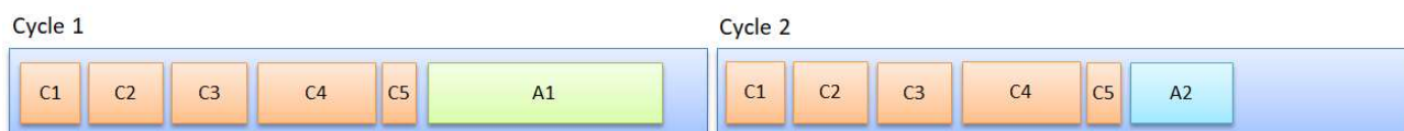
Figure 4: Two network cycles, each showing the same number of cyclic messages with the same amount of data. In both cycles one acyclic message (A1, A2) is sent, with different data.
