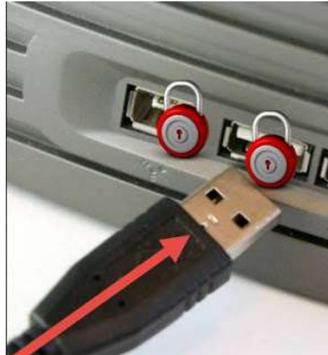
*Figure: Two examples of tools to physically prevent a device or cable to be inserted in a USB-port.*
