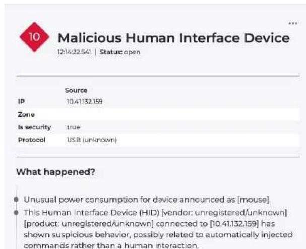
Figure: Detecting malicious USB "HID" devices (source: Nozomi)
