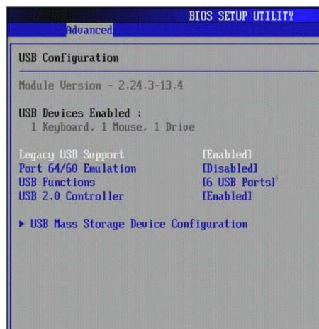
Figure: Disabling USB via a BIOS configuration setting
