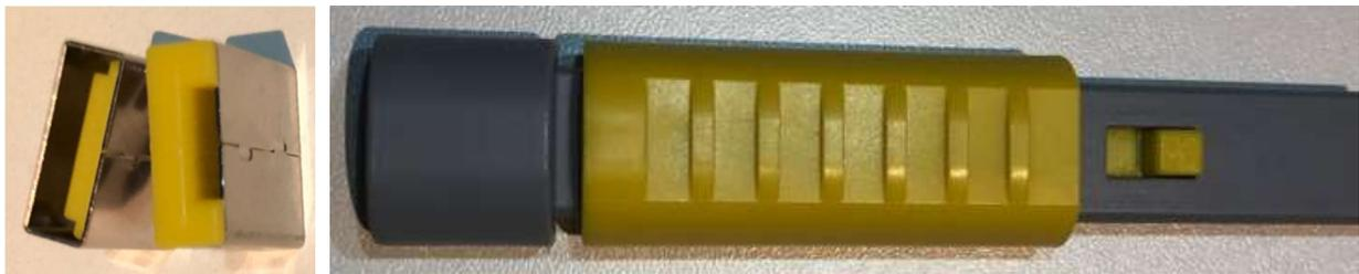
*Figure: USB blocker from SmartKeeper, and the accompanying insertion/extraction tools.*
