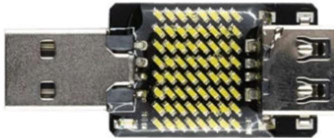
With the yellow LEDs it signals the detection of an overvoltage, and blocks it.
