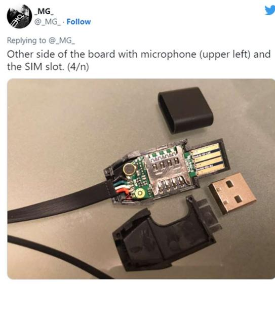
Figure: Spy cable with microphone, GPS and GSM (source: <https://mg.lol/blog/spycable/>)
