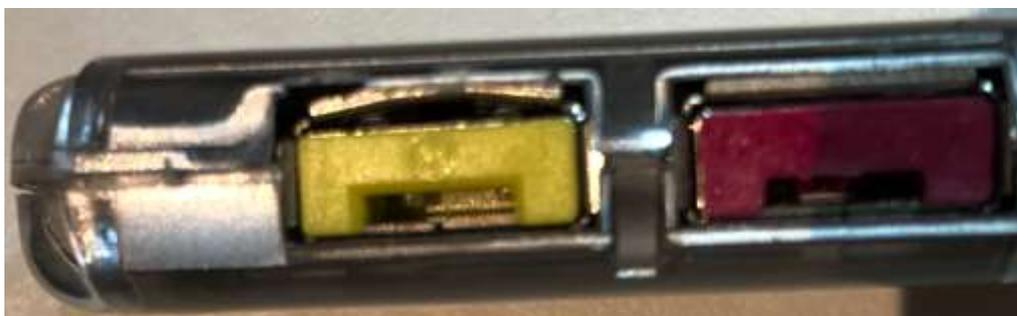
*Figure: damaged USB port after removal of the yellow blocker with a screwdriver.*
