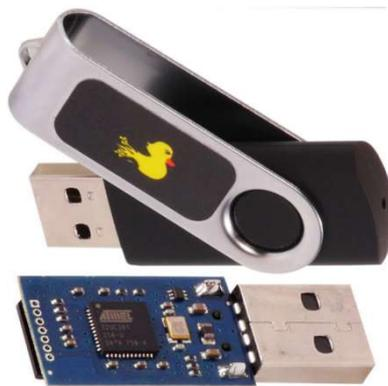
Figure: A "Rubber ducky" in its innocent looking packaging (top), and its internals (below). At the left the slot where an SD-card can be inserted.
