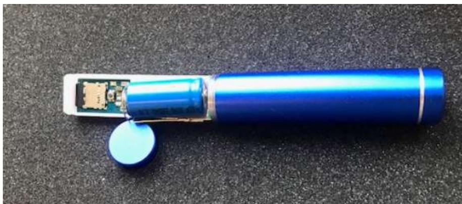
Figure: A rubber ducky inside a power bank. Source: Sepio Systems.
