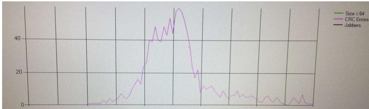
*Figure 1: CRC errors caught with a network tap, as shown by the accompanying software package (source: author)*
