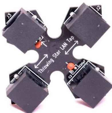
Figure 7: A simple tap, after soldering (source: HakShop)
