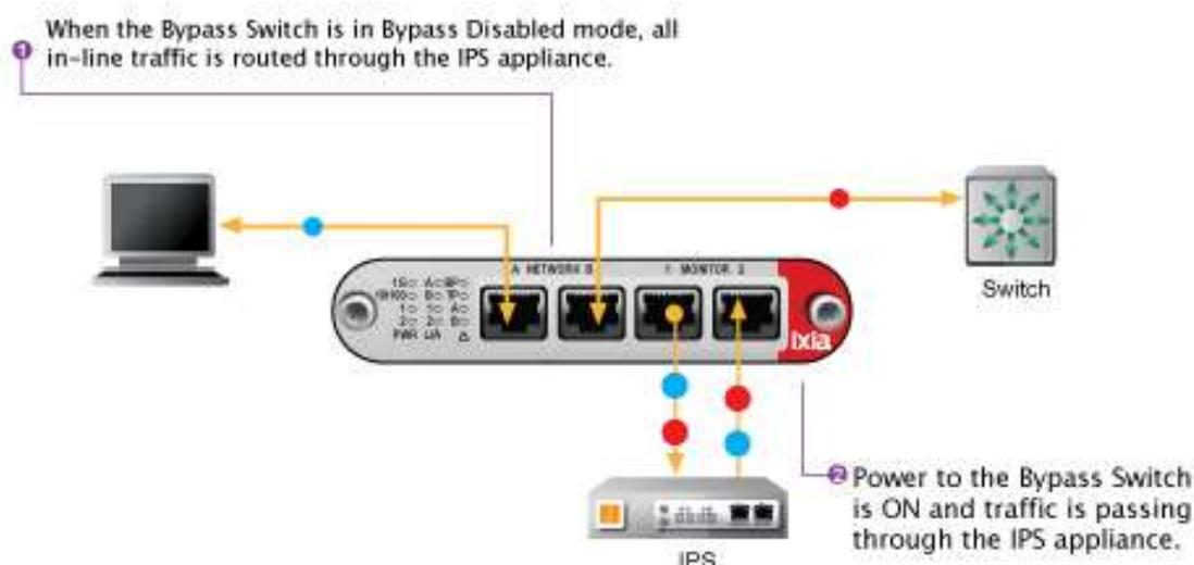
Figure 25: The normal flow of network messages through a bypass tap (source: Ixia)
