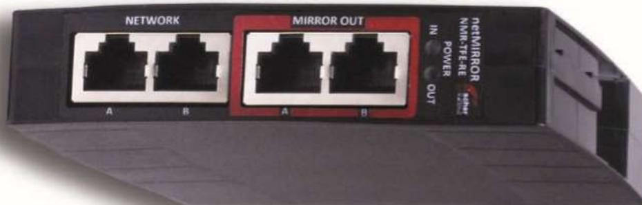
Figure 10: The Hilscher "netMirror" tap (source: Hilscher).
