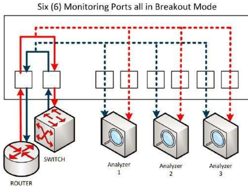
Figure 20: Dataflow in a regeneration tap (source: Garland)
