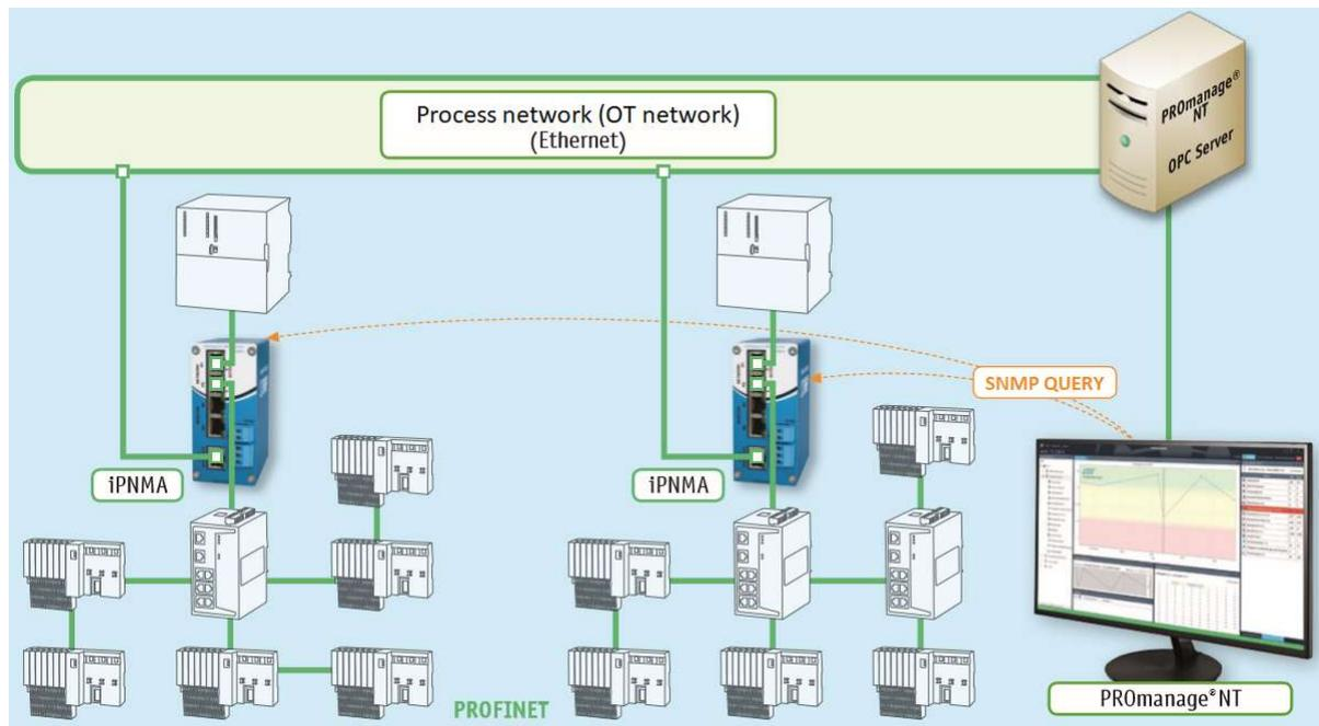
Figure 27: Two InduSol “iPNMA” taps inserted in a ProfiNet system (source: Indu-Sol).
