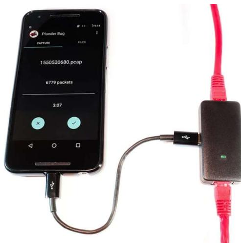
Figure 19: The Hak5 “Plunger Bug” (source: Hak5)
