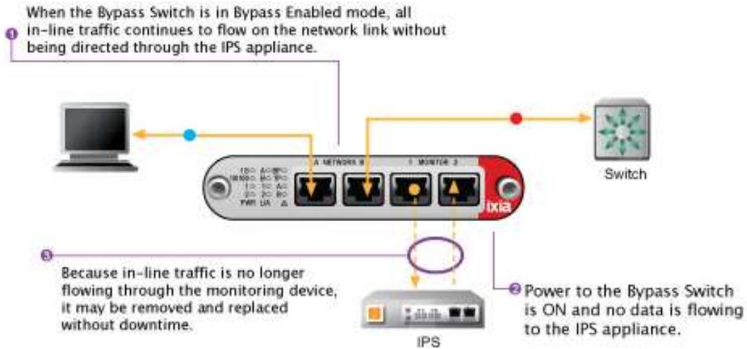
Figure 26: A bypass tap in bypass mode (source: Ixia)
