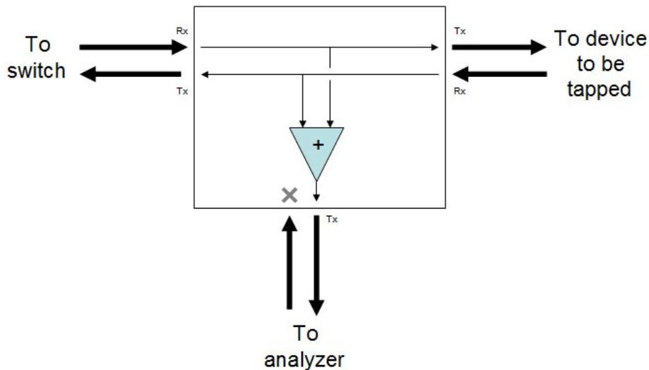
Figure 12: Dataflow in a 100 Mbit/s aggregating tap
