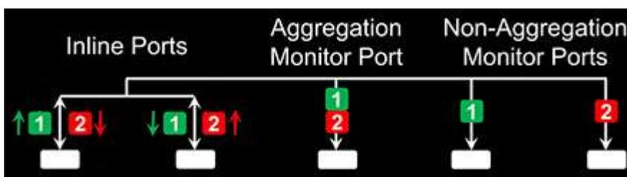
Figure 15: Two data streams combined, or not (source: DualComm)
