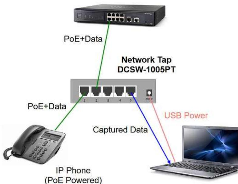
Figure 30: A tap with PoE Pass-through capability (source: DualComm)
