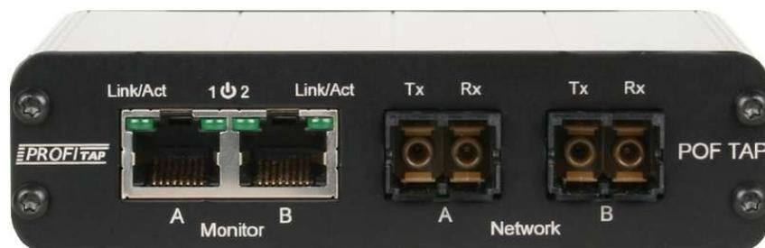
Figure 24: A tap for fiber-optic cabling (source: ProfiTap)
