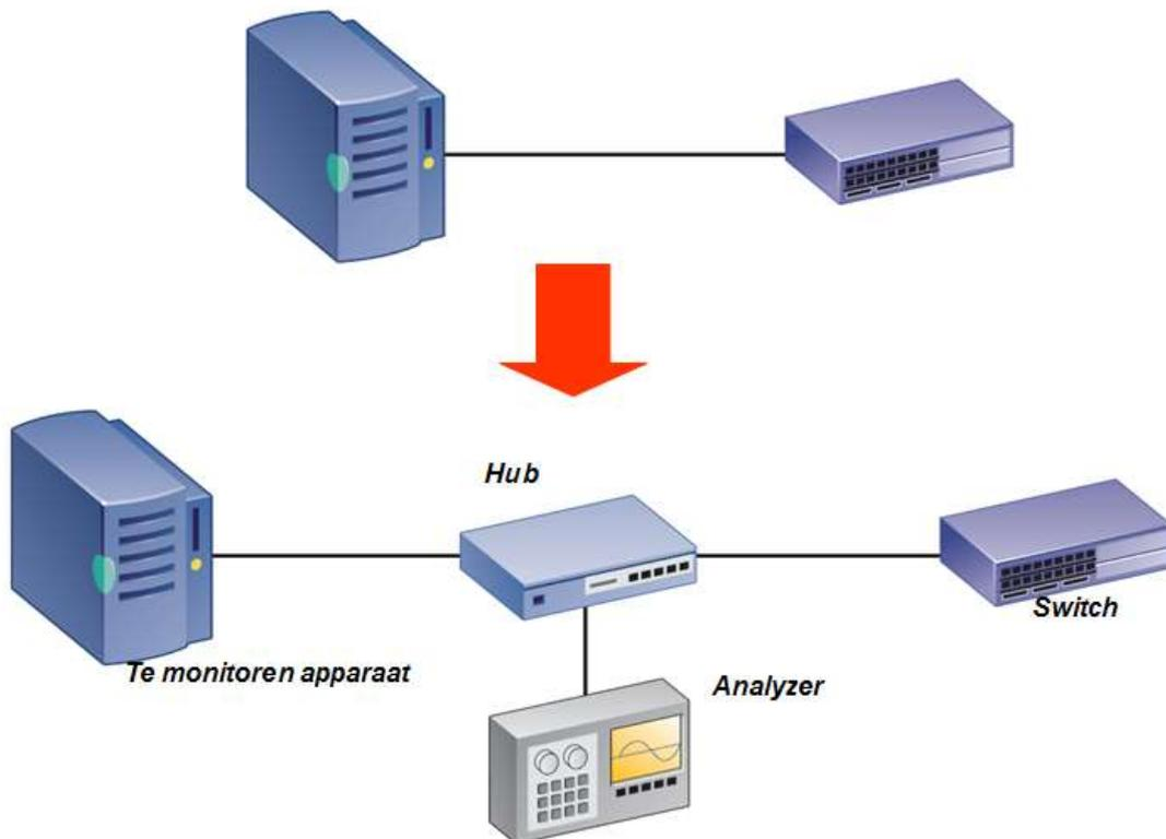
Figure 2: Using a hub to copy network traffic (source: Fluke)
