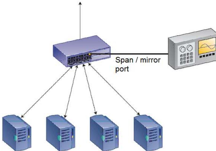
Figure 4: Using a span / mirror port (source: Fluke)
